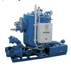
In the Roediger® vacuum station, the wastewater is collected in a wastewater tank and then conveyed with wastewater discharge pumps into a conventional gravity sewer main or directly into a wastewater treatment plant. Vacuum pumps in the vacuum station generate the negative pressure required in the pipe network.
