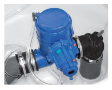
The vacuum valve unit consists of the vacuum valve itself and the corresponding control unit. Roediger® membrane valves are characterised by their durability, universal application possibilities and their simple operation and maintenance. Various valve sizes with internal diameters of 50 mm, 65 mm or 75 mm are available to suit the respective application.
