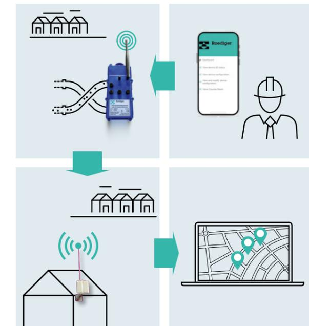
**Backed by proven efficacy, LoRa monitoring seamlessly transmits all vital data wirelessly to a centralized hub. Any irregularities are promptly reported to the operator's smartphone for swift action.**
